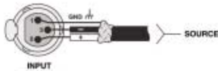
Figure 2.1 Balanced Analog Input Connector Wiring or AES/EBU Digital Connector Wiring
