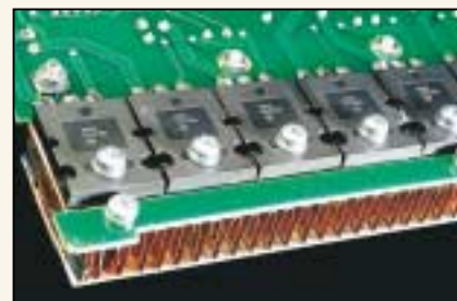
The output transistors are located side-by-side in the airstream
