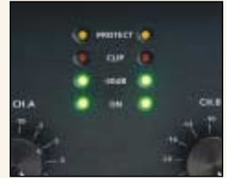
Indicators for VHF and temperature protection.
