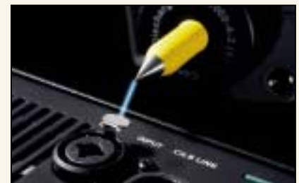
Lab.gruppen's EMC test facilities. 8,000 volts are being "shot" with this gun for testing!
