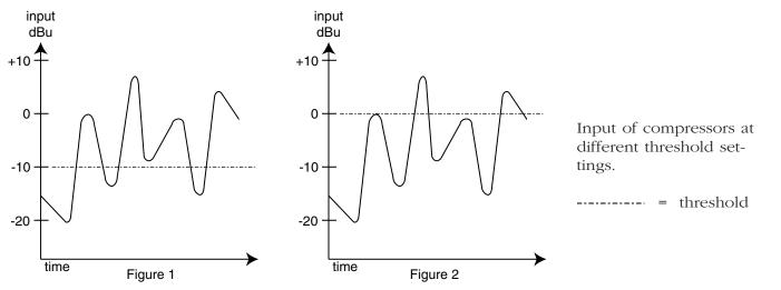
The difference between compression and limiting is shown visually below. In the first diagram below, compression "squashes" the signal. Its peaks are lowered, but the overall level of the signal is raised due to applied make-up gain (Output Gain). In the second diagram, the peaks are lowered to the threshold level, but the rest of the signal has not been altered.
