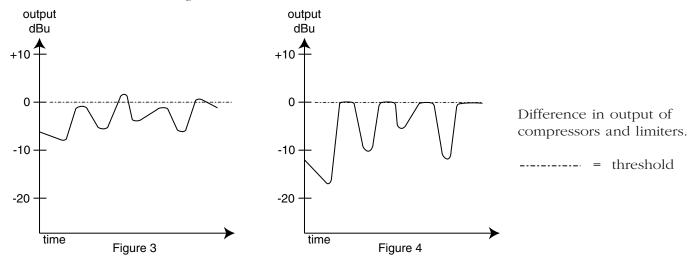
Obviously, there is a large difference between these two signals in relation to their dynamic range and the processed signal. In the third figure, it is shown to have been compressed, and in the fourth figure, it has been limited.
