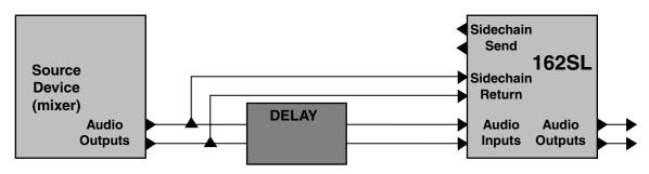
*Common "ducking" setup: delay is inserted into audio input, non-delayed signal fed to sidechain. Sidechain triggers compression before signal is heard.*
