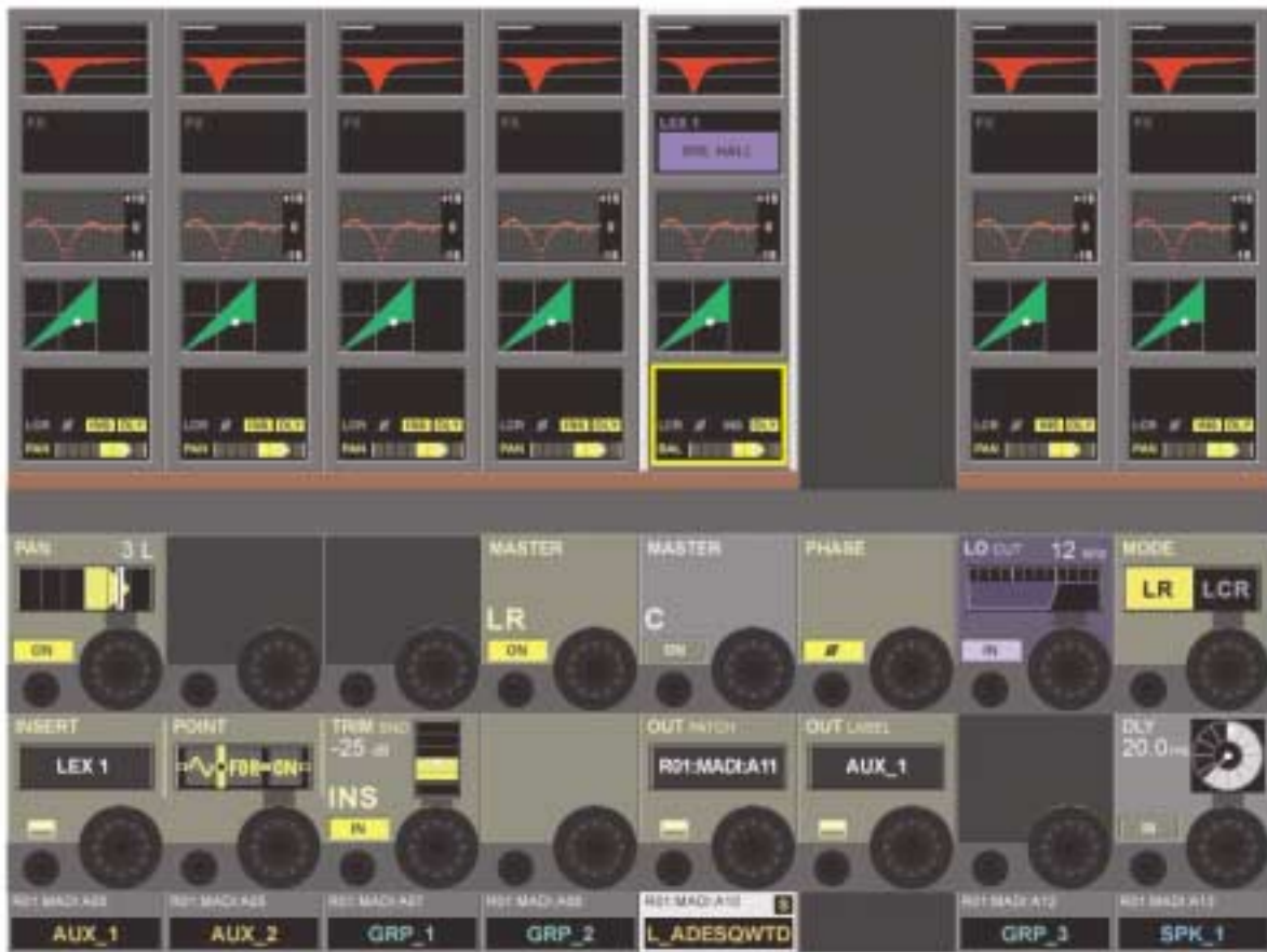
그림 21-8 Selecting An FX Processor As A Master Bus Insert Effect.
