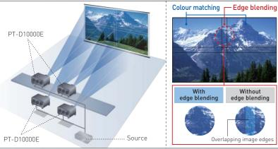
When edge blending and colour matching are set, the brightness and colour balance at the boundaries where screens are joined may lack uniformity due to differences in the uniformity of the screen gain directivity, the brightness of each lamp mode, etc
